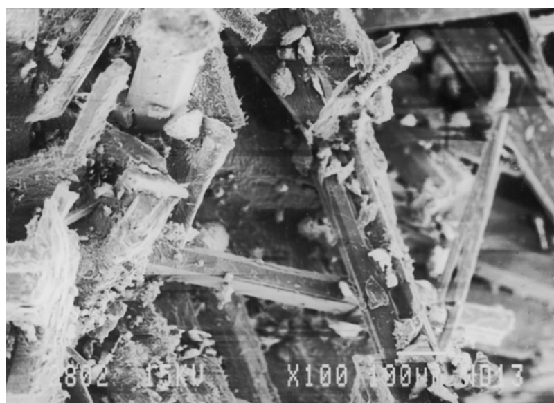
Figure 6 SEM of potassium titanate whiskers formed by the reaction between K_2CO_3 and TiO_2 in TK at 1150°C.
